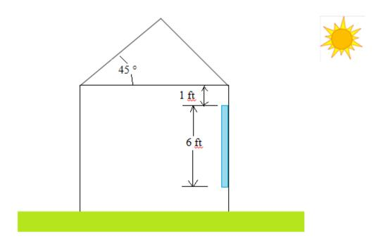
The House above has a roof angle of 45°. It has a southward facing window that is 6 ft tall and 1 ft from the roof top. Assume your design is for Vancouver, WA.
